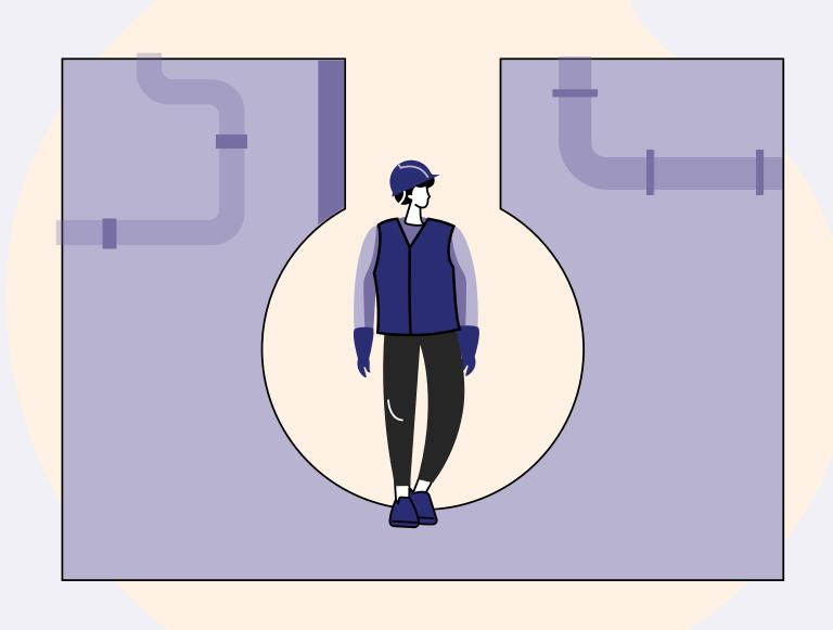
It is vital that we control and monitor the atmosphere. Most confined spaces have one way in/out and awkward or tight means of entry/ egress. ALWAYS have a rescue plan!
