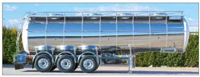
Truck Tanker made of Stainless Steel.
