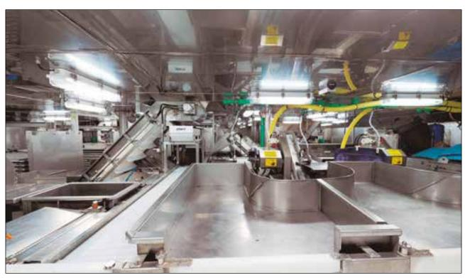
Stainless Steel Machinery for Fish processing, inside a Fishing Boat.
